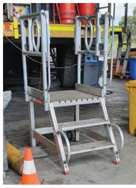
Handles for manoeuverability, Simply lift to engage the front wheels
